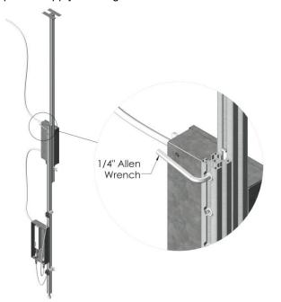
3. Extend the Wired Column by loosening the height adjustment screws and pulling it to the height of the plenum to prepare them for installation. Use a hex wrench to then re-tighten them.
