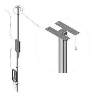
4. Using the appropriate hardware, attach the Vertical Support Bracket to the top of the Plenum.
